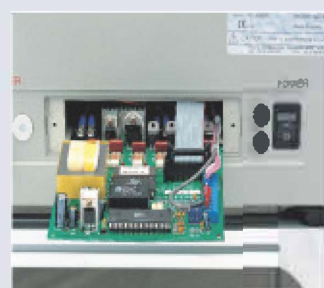
Mainboard on JP-33 All functions controlled by microprocessor on mainboard
